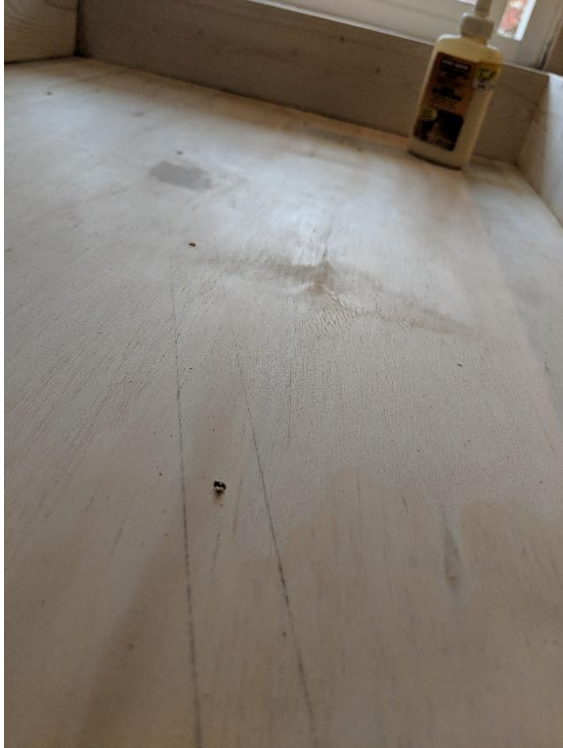
Figure 3: Tracing where each of the pieces sit on the plywood helps to drill the pilot holes.
