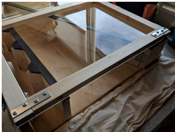
Figure 5: Brackets help strengthen the plexiglass door
