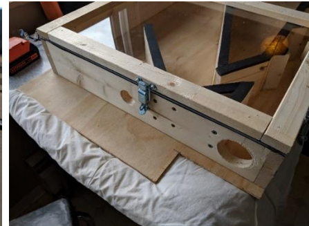
Figure 9: The machine has a single clasp on top, positioned in the centre.
